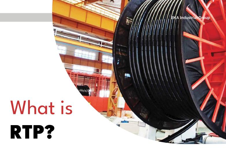
A spoolable composite pipe is a flexible, reinforced thermoplastic pipe made of a thermoplastic liner and one or more reinforcement layers, capable of being coiled for transport and installation.
